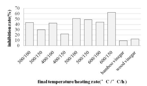
Figure 3 The inhibition rates against Coriolus versicolor of MDF pyrolysis condensate liquids obtained under different pyrolysis conditions
