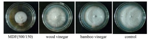
Figure 1 The inhibition effects against Coriolus versicolor of different kinds of pyrolysis condensate liquids
