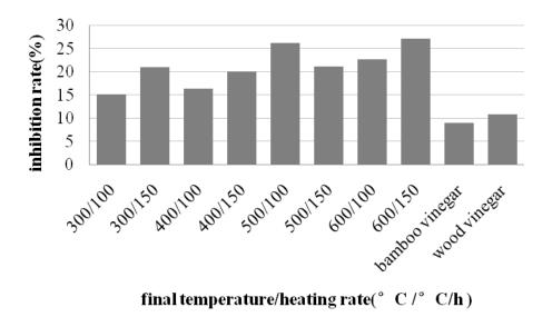
Figure 4 The inhibition rates against Gloeophyllum trabeum of MDF pyrolysis condensate liquids obtained under different pyrolysis conditions
