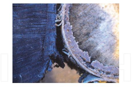
Fig. 9. One cut surface of a birch log (left) was dipped in birch tar oil and photographed after storage for one year outdoors. Many kinds of wood rotting fungi were growing on the untreated cut surface (right) but not on the treated surface.
