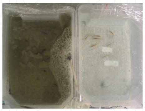
Fig. 12. Test fish swimming in a box treated with birch tar oil (left) and in a control box without birch tar oil (right). No negative impact was recorded on fish although the fish were hardly visible because of the birch tar oil treatment.
